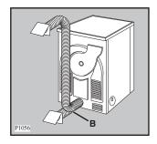
Once connected to the dryer, run the vent hose to the desired outlet point, ensuring that the run's overall length is less than 2 m, and that it contains no more than two bends. As to the outlet itself, if you have decided on a fixed wall/window grille, a good local builder's merchant should be able to supply you with the necessary fittings and installation advice.
