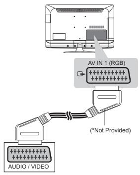
Transmits the video and audio signals from an external device to the TV set. Connect the external device and the TV set with the euro scart cable as shown. To display images by using progressive scan, make sure to use the euro scart cable.
