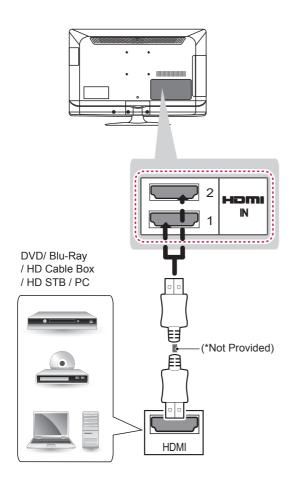
Transmits the digital video and audio signals from an external device to the TV. Connect the external device and the TV with the HDMI cable as shown in the following illustration.
