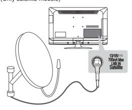
Connect the TV to a satellite dish to a satellite socket with a satellite RF cable (75  $\Omega$ ).
