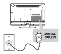
Connect the TV to a wall antenna socket with an RF cable (75  $\Omega$ ).
